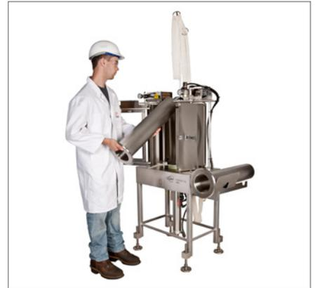
The empty horn is placed into the rucker, mounted onto the lift plate, and secured in place with the locking bar.
