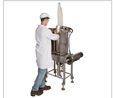
Netting/casing is pulled down over the horn past the grippers (or wheels on some models).
