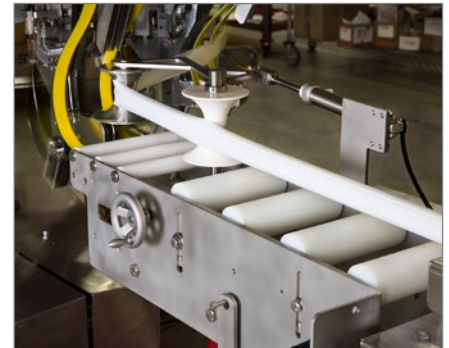
The sealed tube is filled with emulsified product through a constant output pump as it moves to the rotary table.
