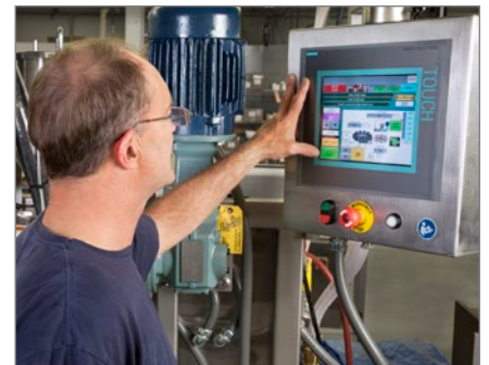
The Human Machine Interface (HMI) touch screen control system makes operation and performance analysis easy and intuitive.
