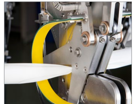
The seal gate gathers the filled tube and securely double clips it.
