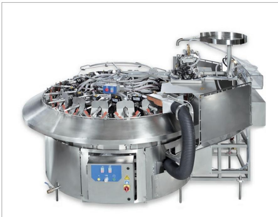
**Rota-Matic** automatic vacuum packaging system for whole birds, pork shoulders, ground meat chubs, rings, loaves, hams and cheese. Operates at speeds up to 40 packages per minute, with 8 or 16 stations.
