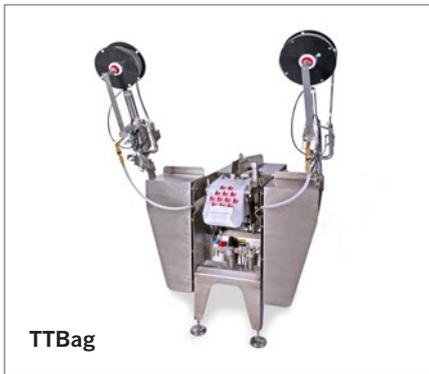
Key traits of the TTBag product line are ease of operation, productivity, and flexibility. The operator pushes the bird through a horn and into a bag, hocks the bird against the hocking station, twists and clips the bag with an optional Econo Clipper or Signature Series clipper.
