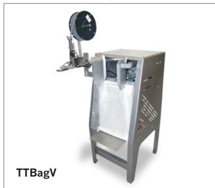
horizontal Signature Series clipper. With a single operator, the TTBag and TTBagV achieve throughput rates up to 20 packages per minute while bagging, or 10 packages per minute for bagging and clipping. Capacity is doubled on the TTBag with the addition of a second hocking station and clipper, and an additional operator.
