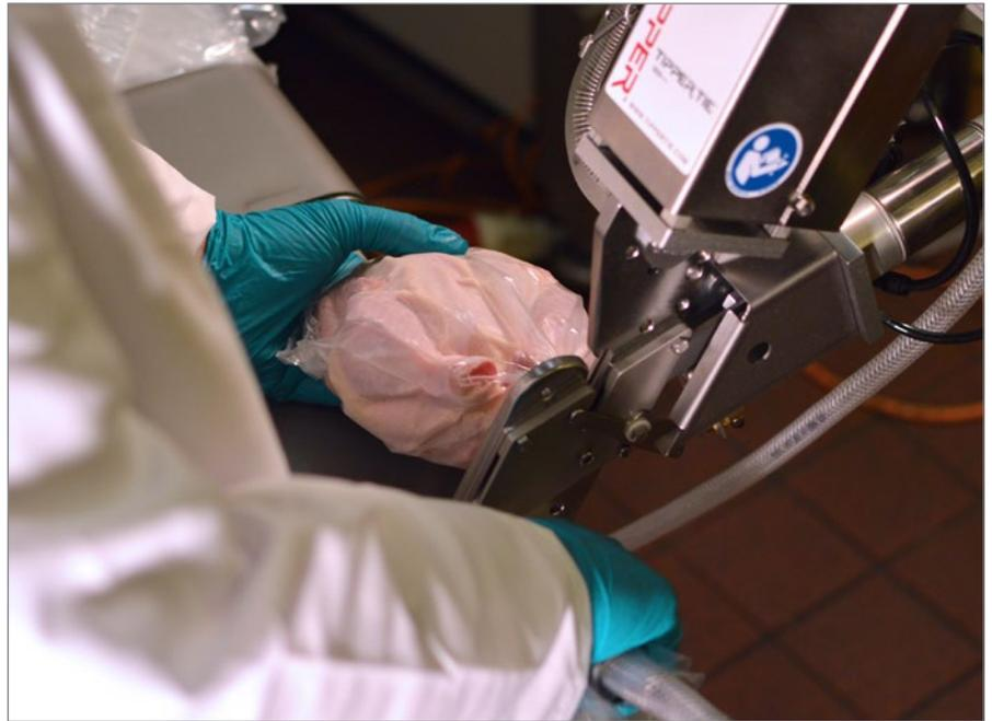
Vacuum sealed bagged poultry from the TTBagS ready for the shrink tunnel.
